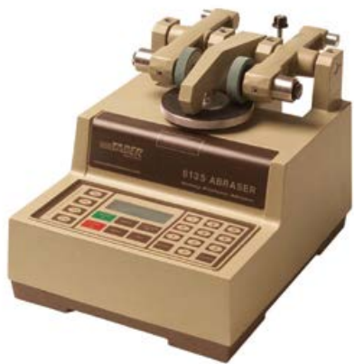
The Taber abrasion meter is a laboratory instrument for measuring abrasion resistance by rotational rubbing of many materials, including wood.
